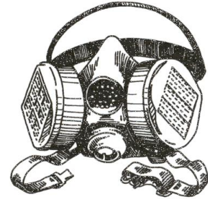
Air-purifying half-mask respirator equipped with P100 cartridges
