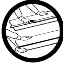
Cutting asbestos-containing wall board by hand
